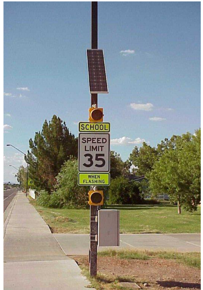
Solar-powered school zone flasher runs daily from 7 a.m. to 4 p.m.
