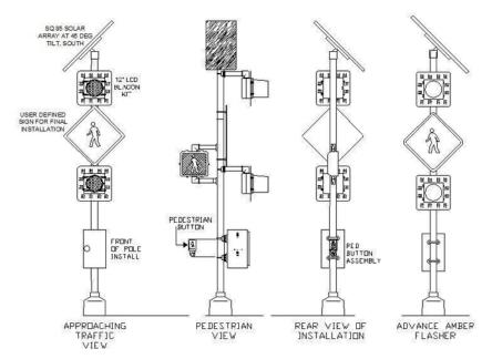
and the DW remains solid. A field adjustable "red clear" timer was the first timing interval to run and was included to allow cars to come to a stop at the crosswalk prior to walk interval. This timer is field programmable from 3 to 20 seconds depending on vehicle speeds.
