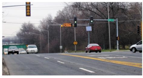
"Viaduct Flodded" flashes on Solar Traffic Controls advanced high-water flasher warning system which incorporates features suchas the ability to call the user with a verbal message announcing an alarm; also to email, fax and page. Uses Motorola police radios to pass the "on" command from the sensor stations to a combiantion of flasher-variable message signs.
