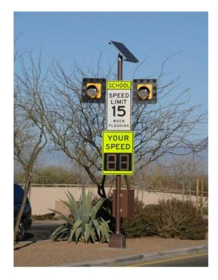
The display characters are 15-inches allowing good visibility to motorists. To aid enforcement of the school speed limit the systems were equipped with 2.5-inch confirmation lamps at the rear of the assembly which face into the school zone. The confirmation lamp allows police officers to see when the 12-inch lamps are flashing and the speed limit is reduced.
