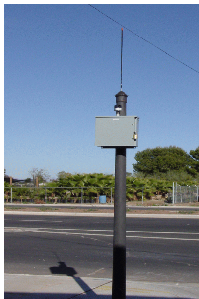
Figure 4 - Optical detector unit with radio transmitter package
